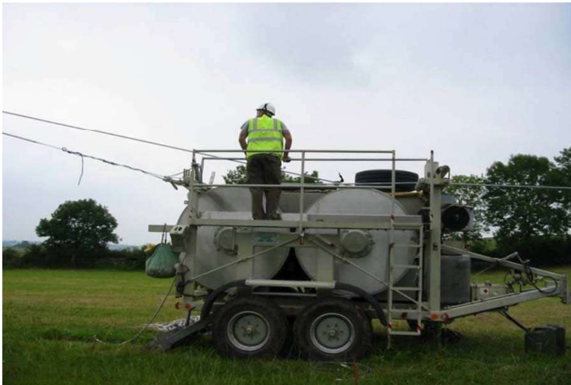
Figure 2.5 Puller – Tensioner machine
